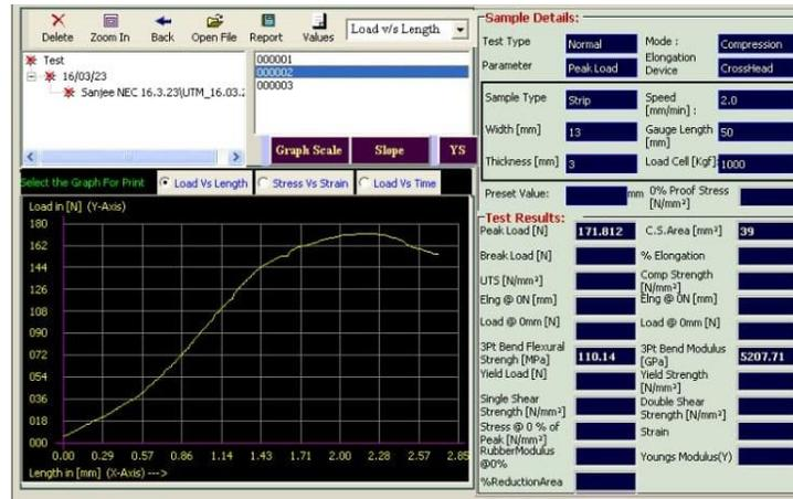
Figure 9. Flexural modulus of CF/PP composites
