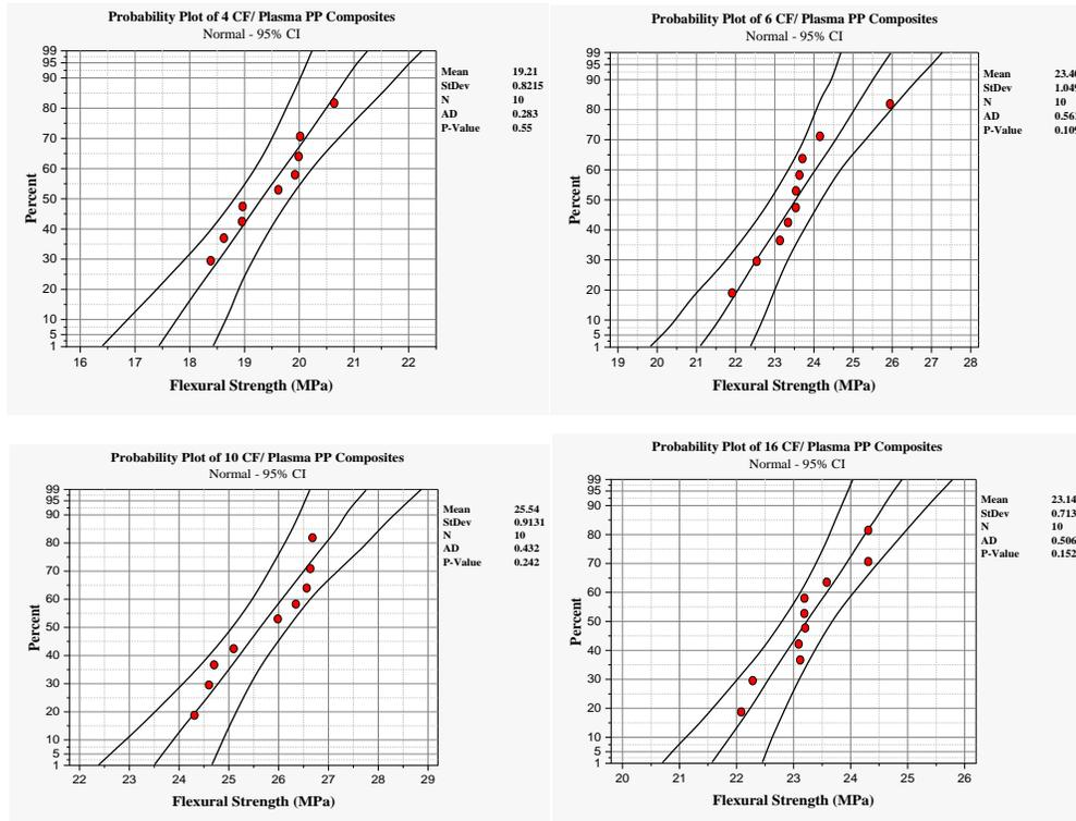
Figure 8. Normal probability plot for FS: (a) 4% Carbon Fiber/plasma PP, (b) 6% CarbFiber /plasma PP, (c) 10% Carbon Fiber /plasma PP and (d) 16% Carbon Fiber /plasma PP combinations.
