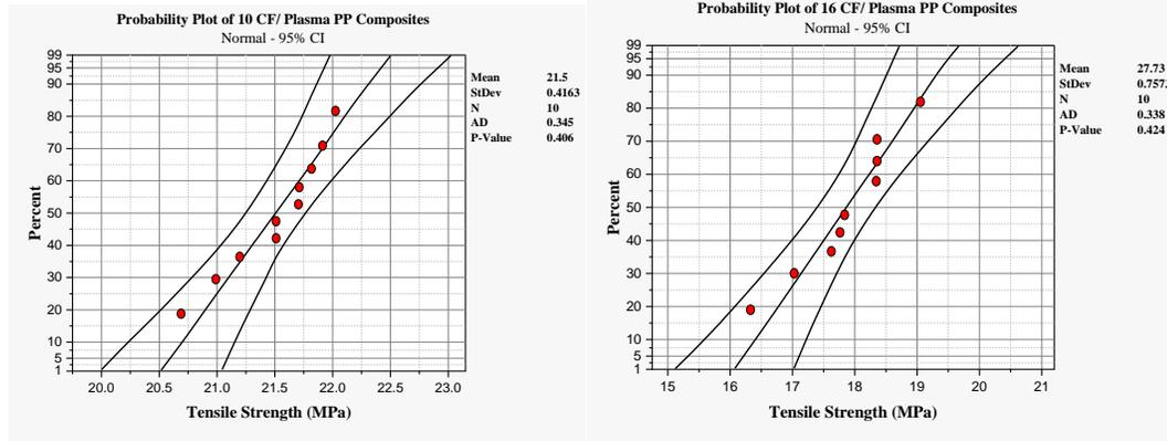
**Figure 3. Normal probability plot for TS: (a) 4% Carbon Fiber/plasma PP, (b) 6% Carbon Fiber /plasma PP, (c) 10% Carbon Fiber /plasma PP and (d) 16% Carbon Fiber /plasma PP combinations.**
